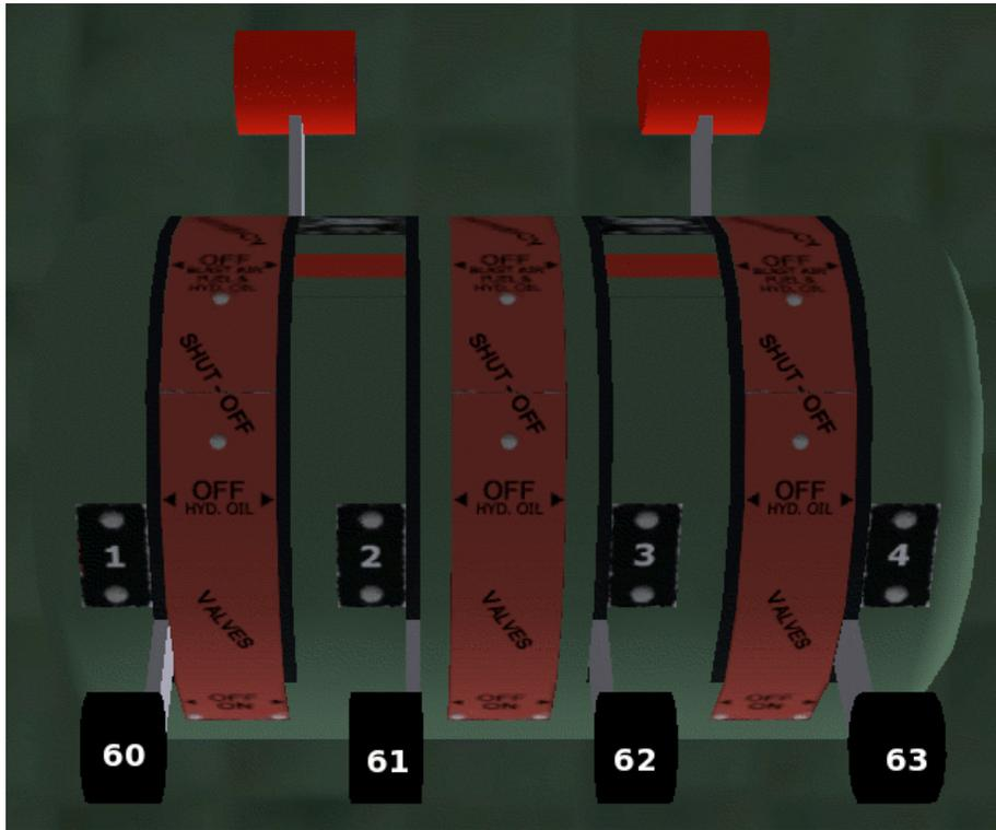
*Figure 14 - the Overhead Engine Cut-Off Drum*
