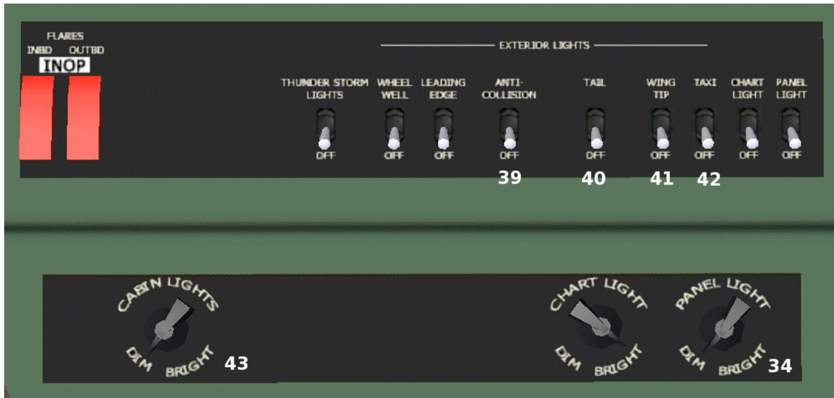
*Figure 11 - the pilot's left side electrical panel*
