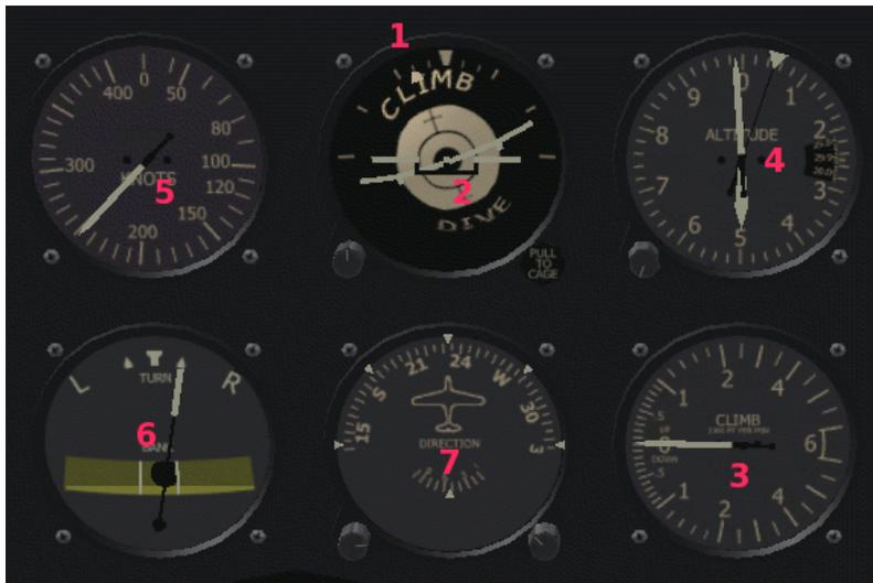
In the instrument cluster detail to the left, the 6 key instruments are shown while executing a right turn at 5000 feet. The numbers correspond to the following points:
