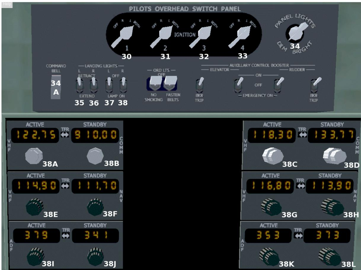
Figure 10 - the pilot's overhead switch panel
